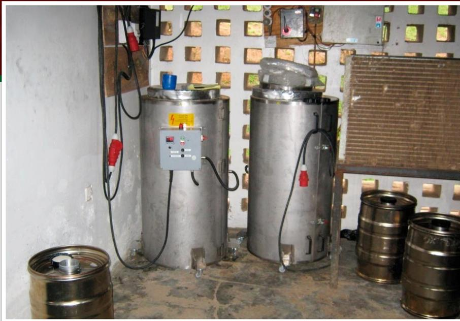
CoolChurn (left): Height = 560 cm; Diameter = 380 cm, Milk capacity = 15.5 liters; Weight, empty = 22.0 kg; Weight, full = 37.5 kg; Opening diameter = 9.0 cm. A pair of electric regenerator installed at the collection center (right). Each unit regenerates two stacked-up coolers.
